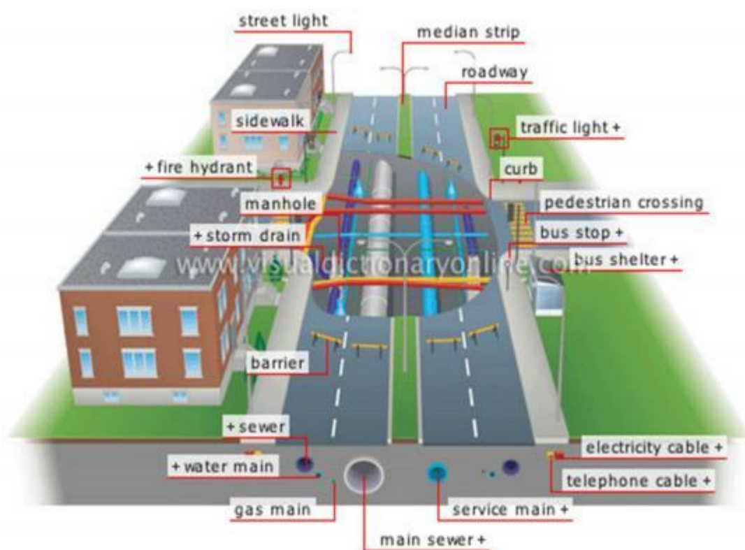
Figure 14. A built-up modern road with integrated infrastructure for water, sewer, electricity and telecommunications facilities.
